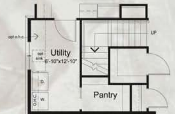
Utility Room on Crawl with Bonus Room
